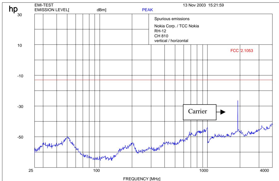
**$f < 1 \text{ GHz}$  : RBW/VBW: 100 kHz** **$f \geq 1 \text{ GHz}$  : RBW / VBW 1 MHz****Carrier suppressed with a rejection filter****REFERENCE NUMBER(S) OF TEST EQUIPMENT USED**
