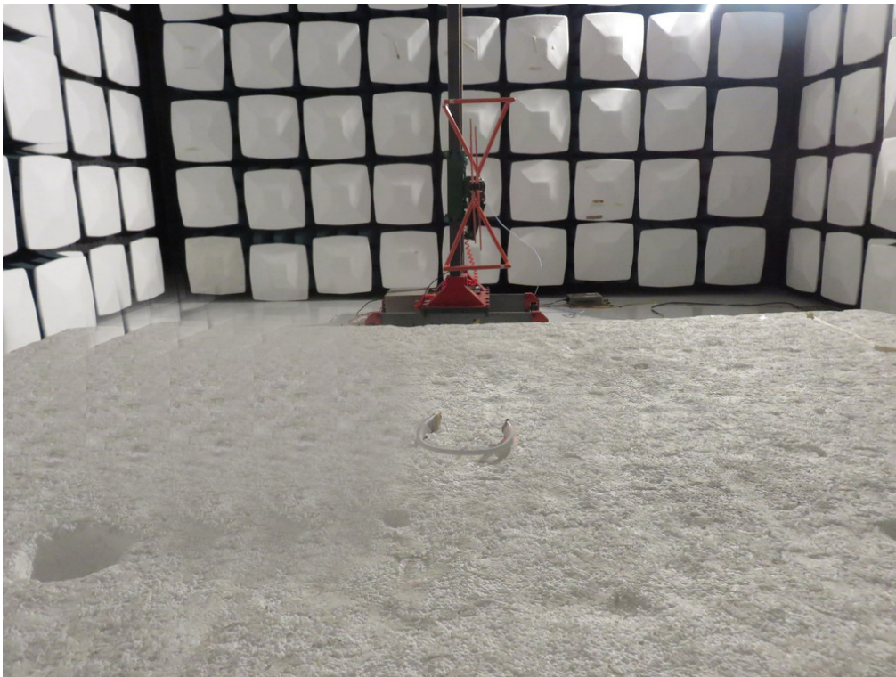
FCC RADIATED EMISSION TEST SETUP
