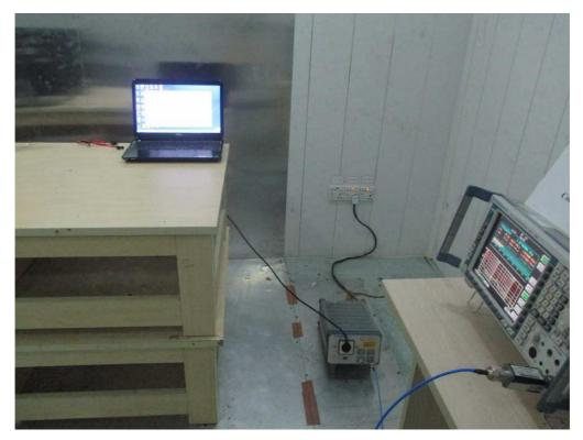
FCC RADIATED EMISSION TEST SETUP
