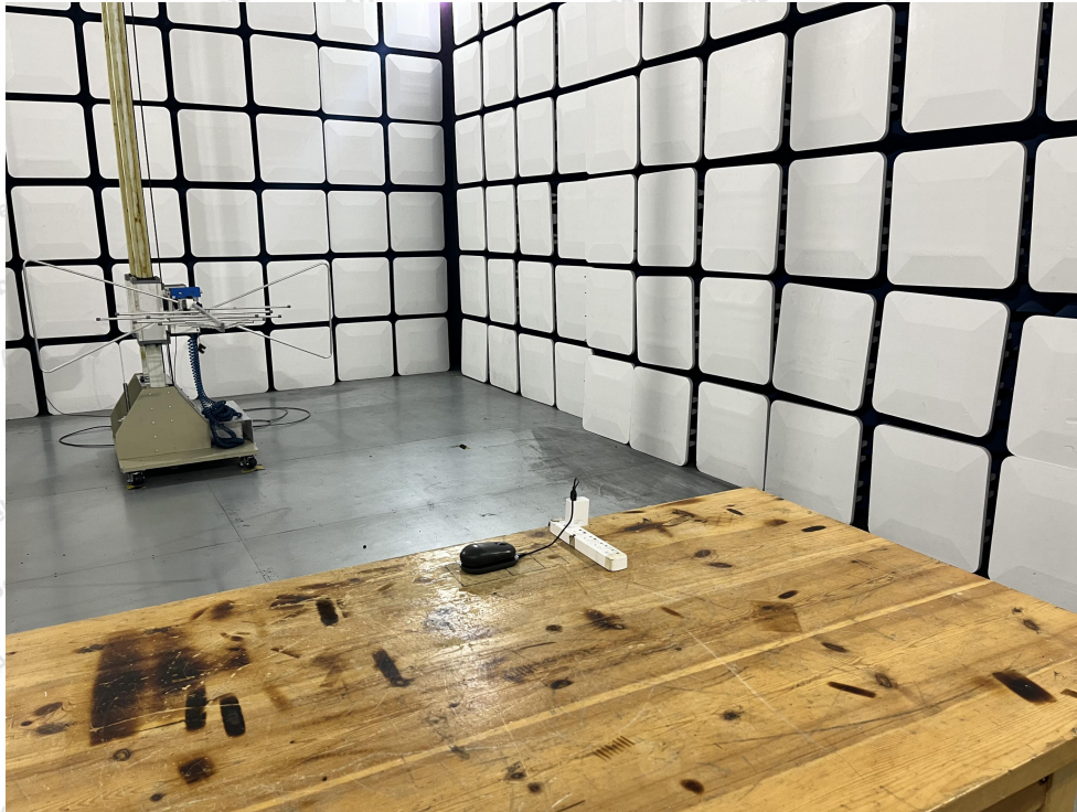
Photo of Radiation Emission Test
