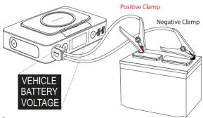
NOTE: Do not touch red (positive) and black (negative) clamps together at any point. If the jump-start button flashes and the 'SAFETY CHECK FAIL' indicator is visible on the digital display screen, the jumper cables have been connected incorrectly. If this flashing red condition occurs, disconnect the jumper cables from the mophie powerstation go wireless and the vehicle battery and restart the process from Step 1.
