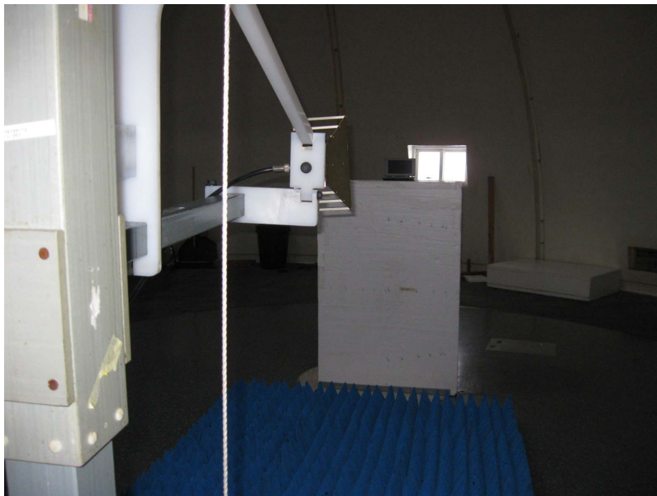
Test Set Up ( Horizontal- DRG ) (Bore-sight antenna)
