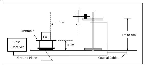
(c) For radiated emissions above 1000MHz
