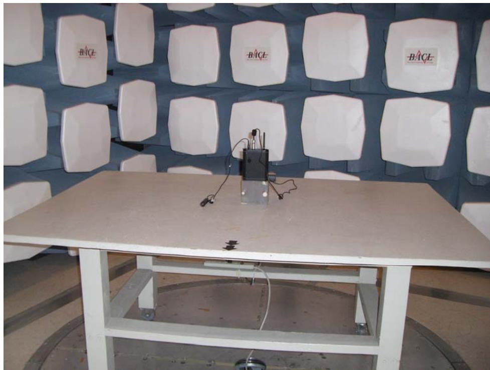
**11.6 Transmitter Radiated Spurious Emissions – Rear View**
