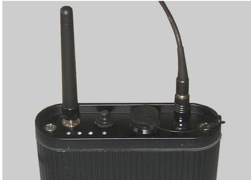
**Figure 3. Attaching the supplied antenna**
