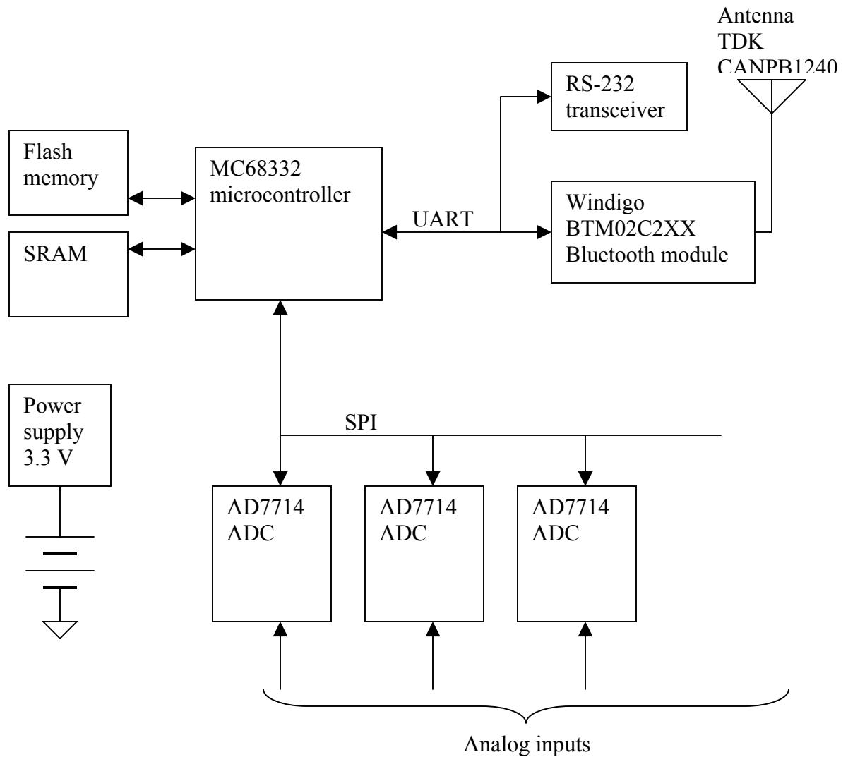
Figure 1. Block diagram of the wireless ISIS (battery power option).
