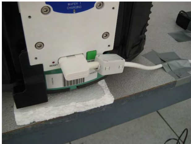
Modification 1: Ferrite, Wurtz electronics, 742.711.32
