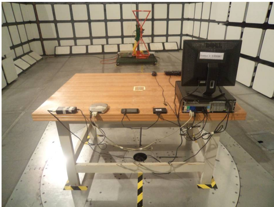
Radiated Emissions – Rear View (Below 1 GHz)
