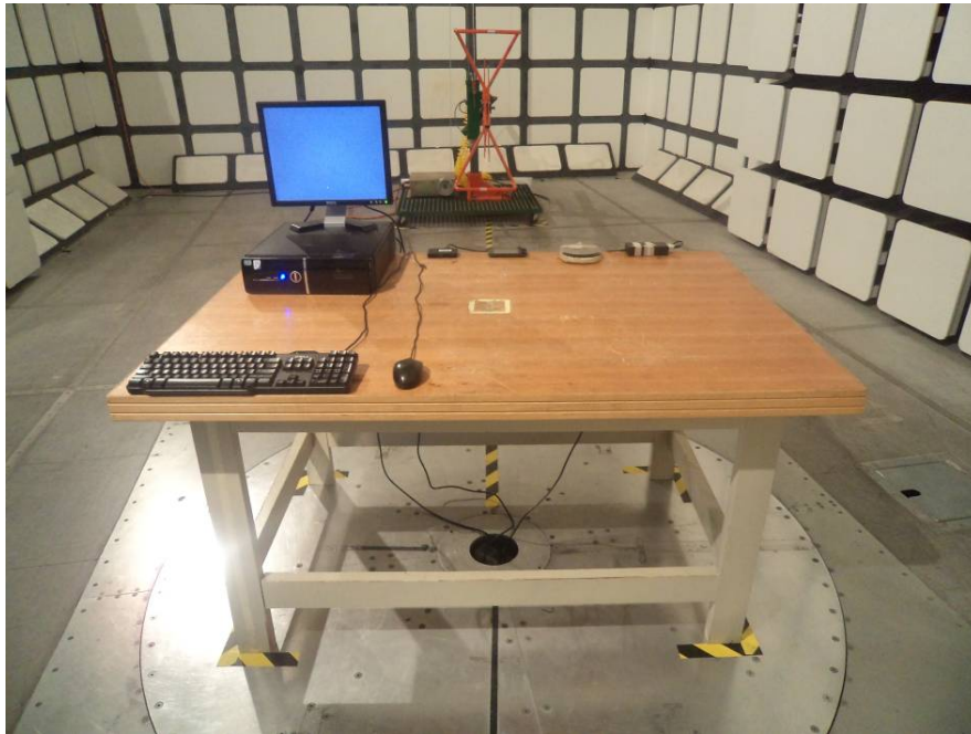
Radiated Emissions – Front View (Below 1 GHz)
