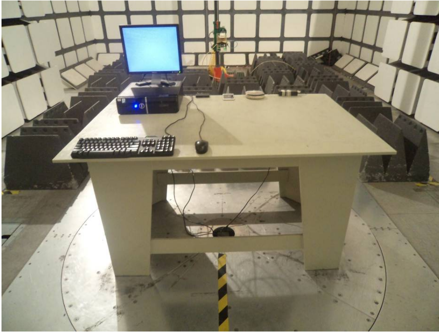
Radiated Emissions – Front View (Above 1 GHz)
