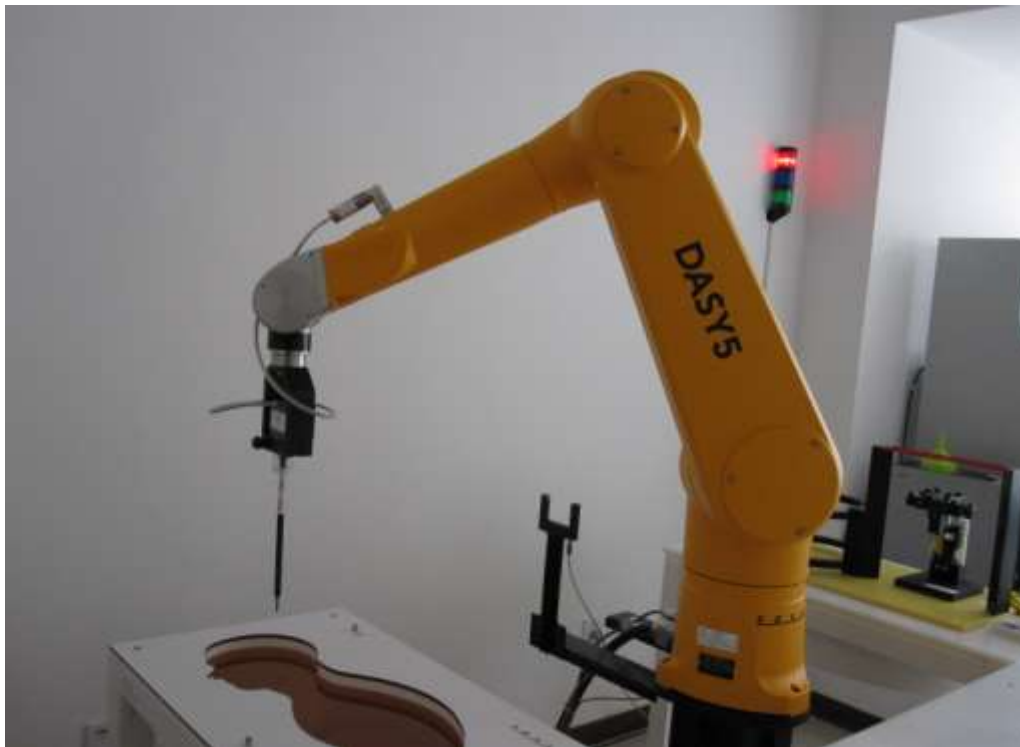
Picture C.1: Specific Absorption Rate Test Layout
