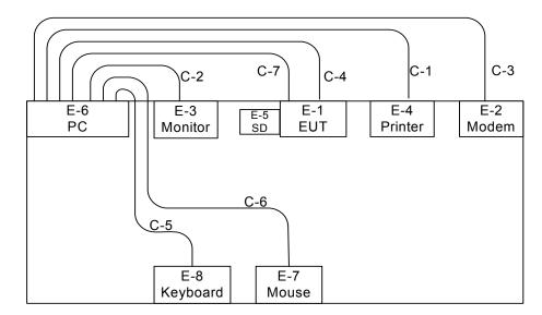
C-1: Parallel Cable C-2: D-Sub Cable C-3: RS232 Cable C-4: USB Cable C-5: USB Cable C-6: USB Cable C-7: RJ45 Cable
