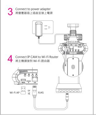
3 minutes to activate after power on then the LED indicator turns to blue 啟動電源 3 分鐘後 LED 指示燈變成藍色
