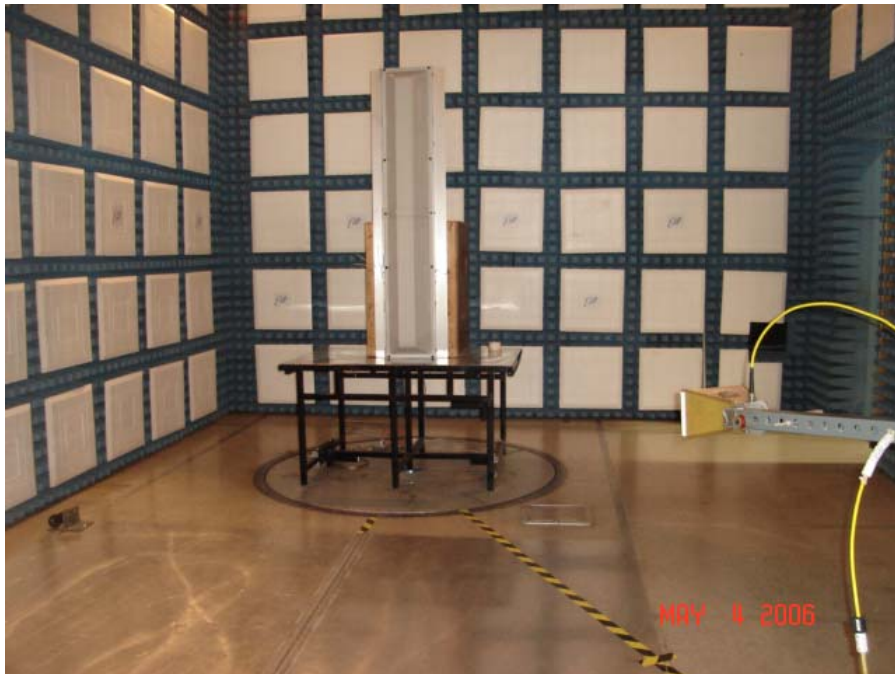
Test Setup For Measurement of Radiated Emissions Vertical Polarity
