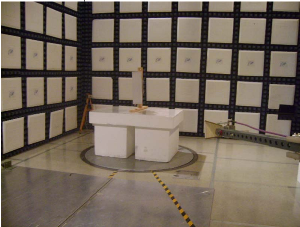
Test Setup for Radiated Emissions Vertical Polarization
