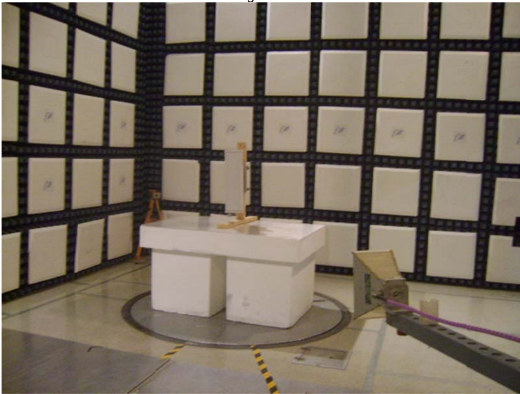
Test Setup for Radiated Emissions Horizontal Polarization
