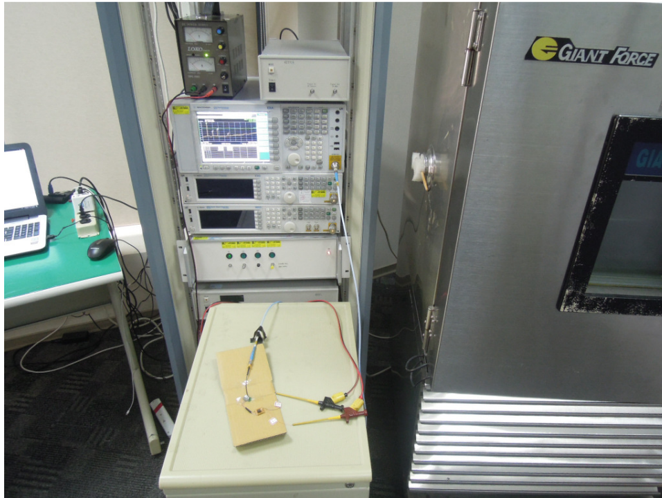
Photograph 6: Set-up for Conducted testing
