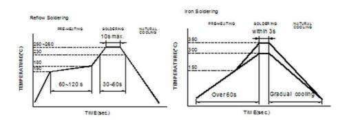
Recommended temperature profiles for re-flow soldering in Figure 1.
