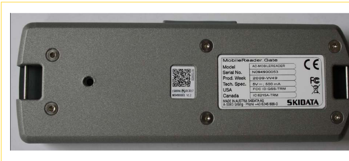
Fig. 2: AC-MOBILEREADER rear view
