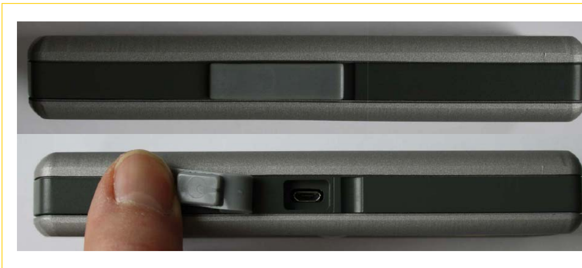
Fig. 4: AC-MOBILEREADER side view (with USB jack)
