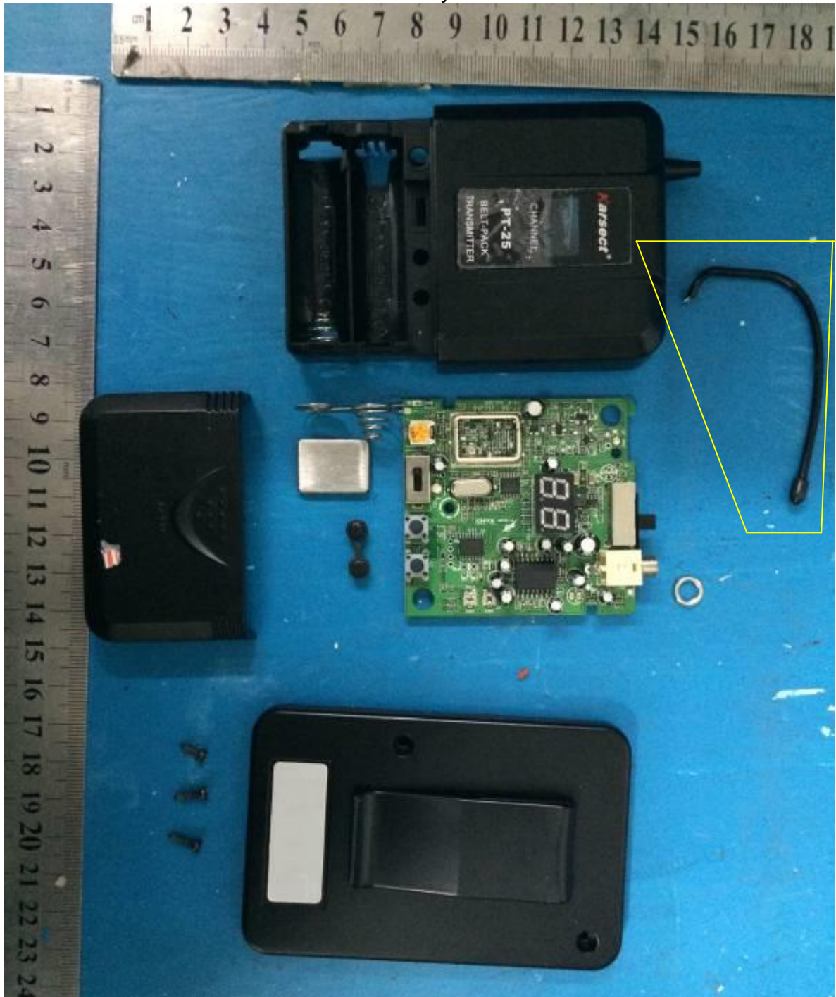
PT-25 with PCB Layout's Antenna
