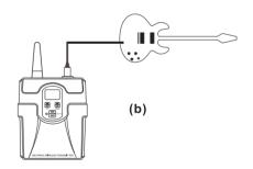
4. Transmitter Battery Installation: Open the battery cover and insert two AA (1.5V) Alkaline batteries. (Att. the battery polarity)
