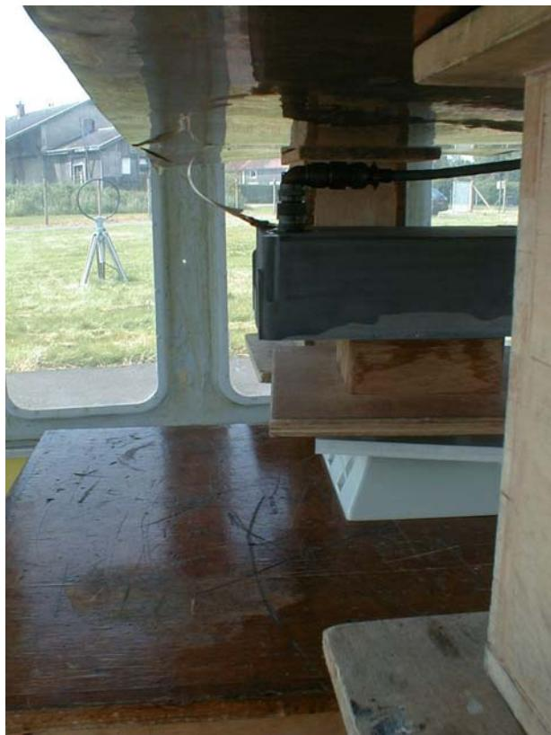
The standard ANSI C63-4 authorizes to realize the measurement in an open site without ground plane under the antenna at the frequencies inferior to 30 MHz.
