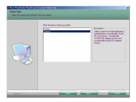
**Step 5.** Choose the "Custom" installation. You can select "Application (WLAN Monitor)" components only and click on "Next".
