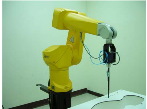
Fig. 5.2 Probe setup on robot
