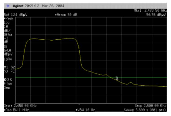
Detector mode: Peak Polarity: Horizontal
