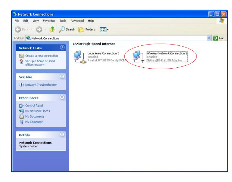
5.Select a pair **Network** icon and click the right bottom of mouse. Then select "Bridge Connections" to create a network bridge
