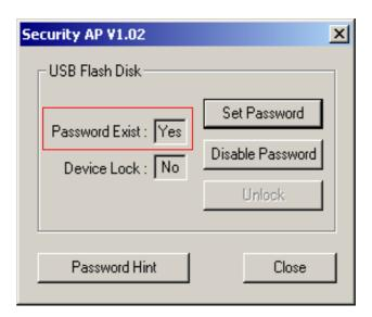
8. Unplug and plug the device again, the HDD partition of the device is locked automatically. It is not accessible until you "UNLOCK" it with the "Security" software.
