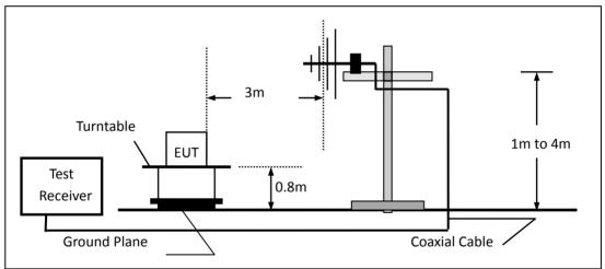
(c) For radiated emissions above 1000MHz
