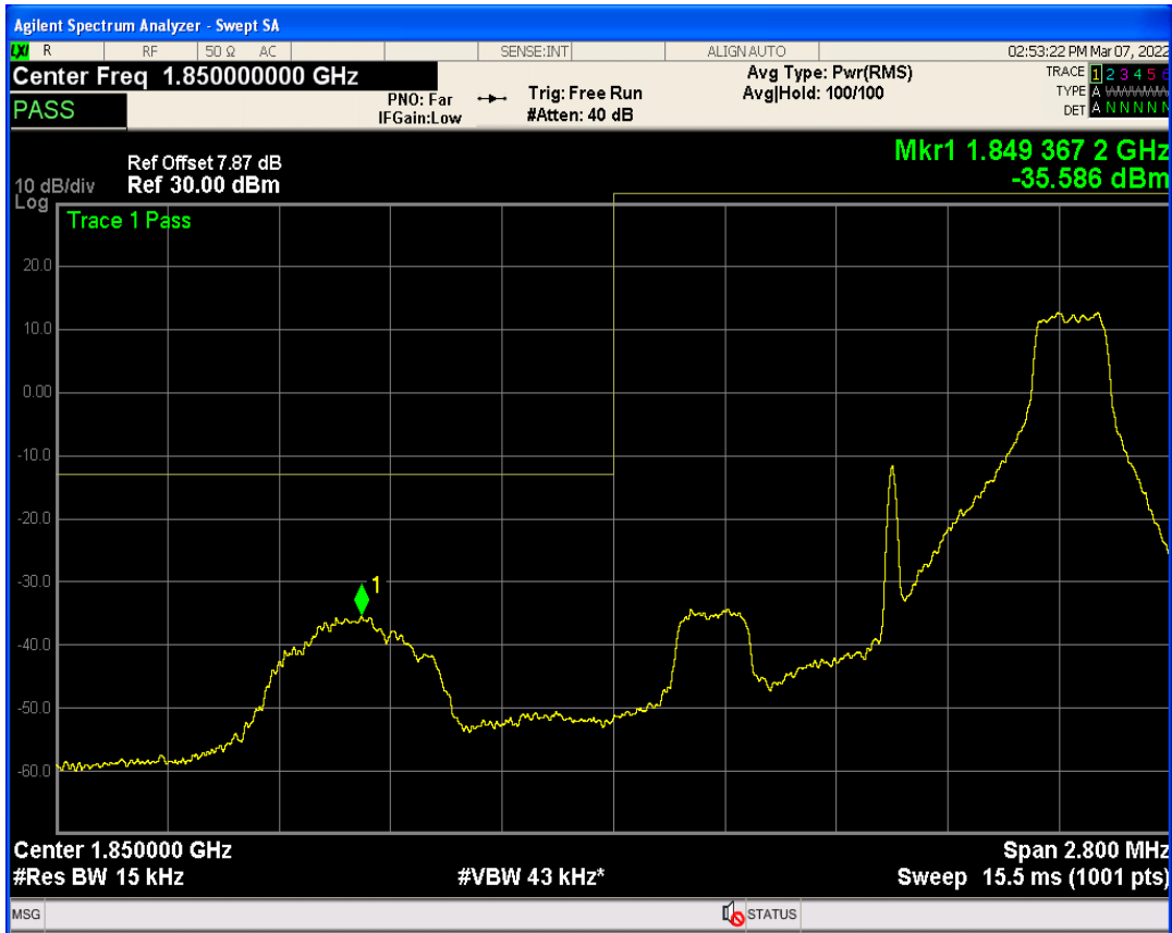
Band2 QPSK BW=1.4MHz Channel=18607 RB Size=1 Position=#0
