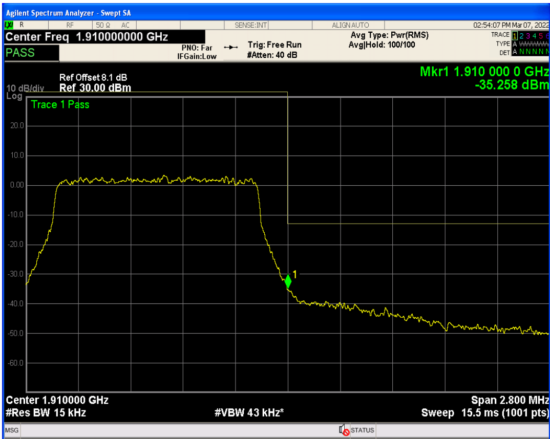
Band2 QPSK BW=3MHz Channel=18615 RB Size=1 Position=#Max
