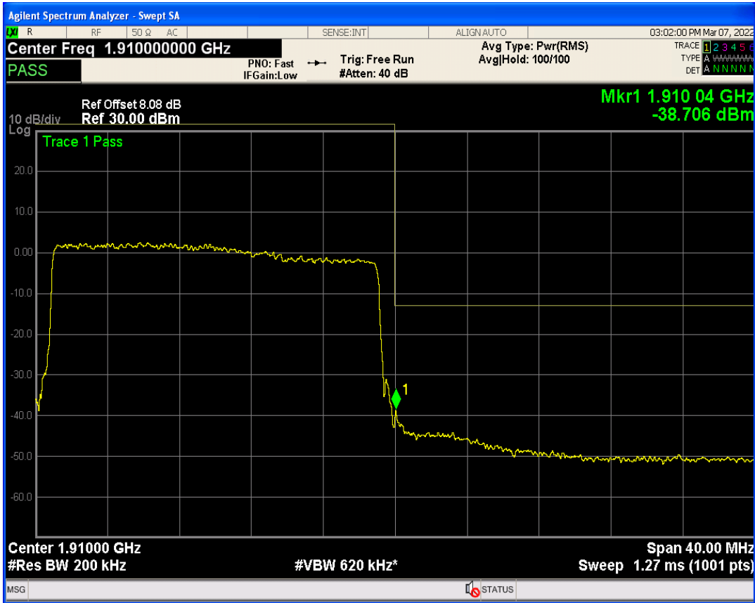
Band4 QPSK BW=1.4MHz Channel=19957 RB Size=1 Position=#0
