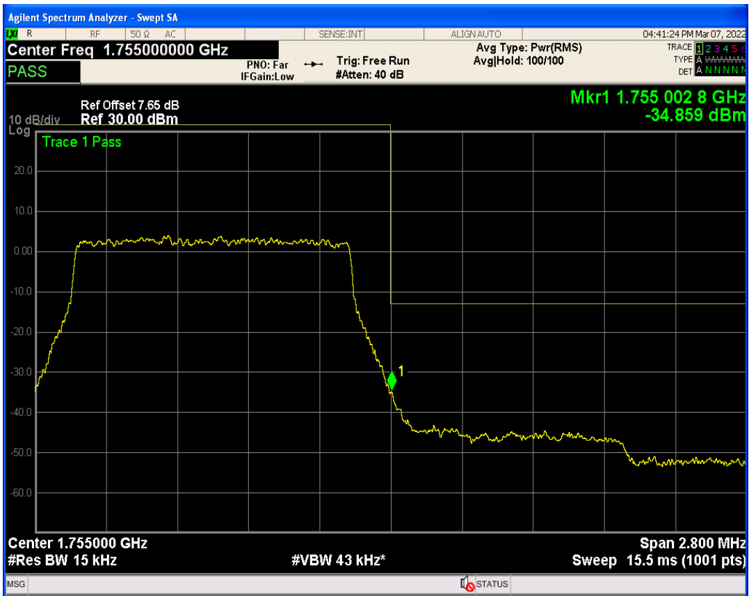
Band4 QAM16 BW=1.4MHz Channel=20393 RB Size=1 Position=#0
