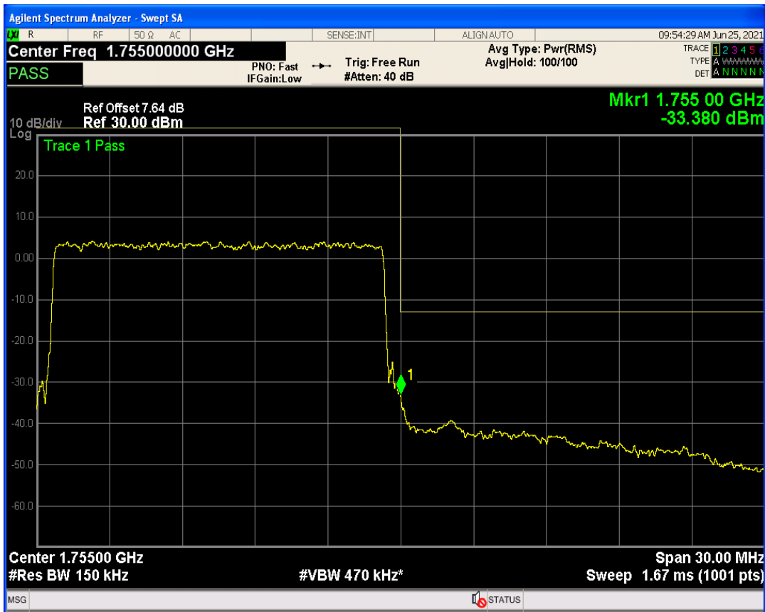
Band4 QAM16 BW=15MHz Channel=20325 RB Size=1 Position=#Max
