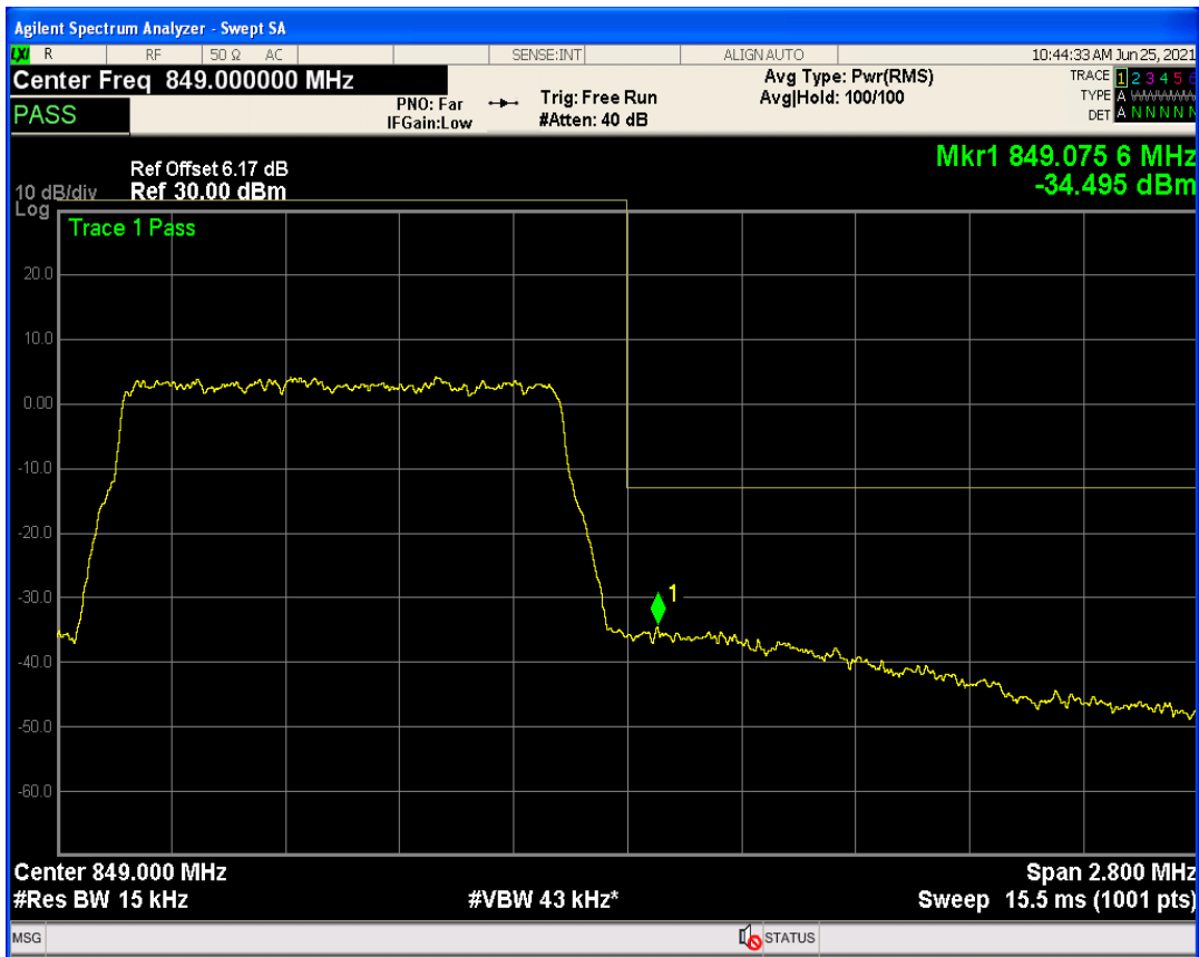
Band5 QPSK BW=3MHz Channel=20415 RB Size=1 Position=#Max
