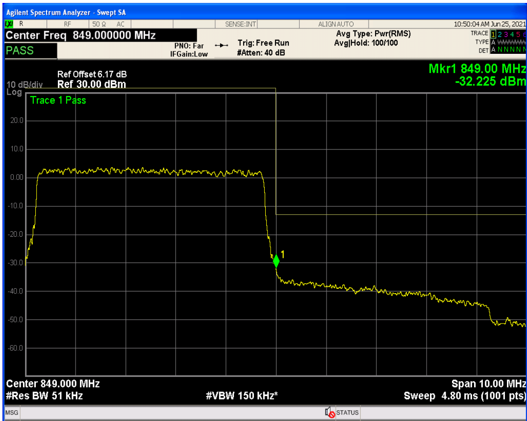
Band5 QAM16 BW=5MHz Channel=20625 RB Size=1 Position=#0
