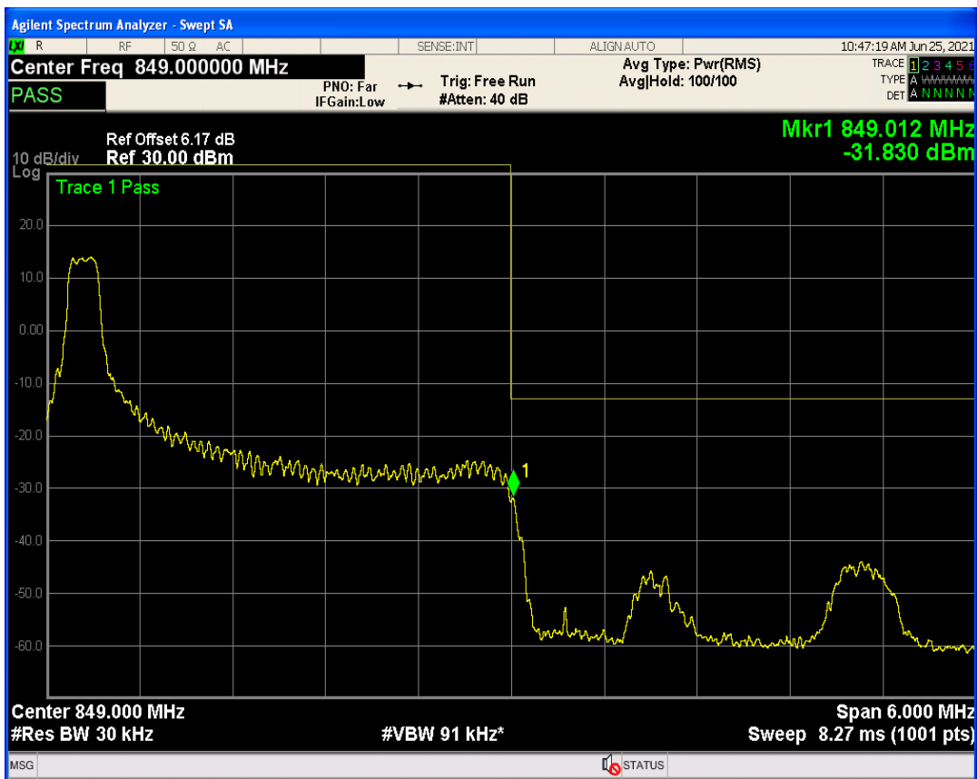
Band5 QAM16 BW=3MHz Channel=20635 RB Size=15 Position=#0
