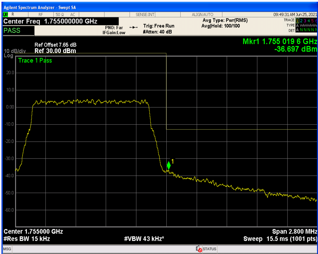
Band4 QAM16 BW=1.4MHz Channel=20393 RB Size=1 Position=#Max
