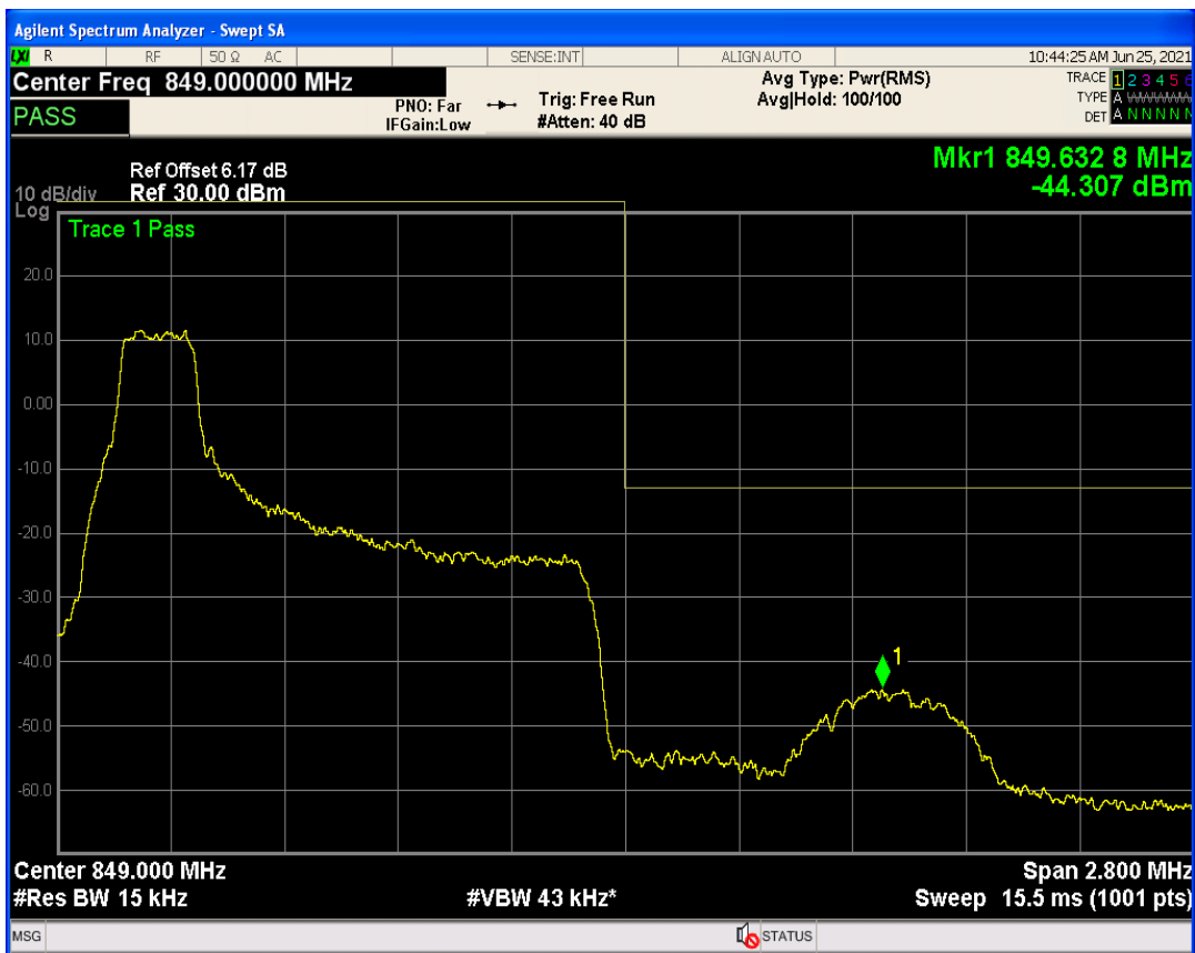
Band5 QAM16 BW=1.4MHz Channel=20643 RB Size=1 Position=#Max
