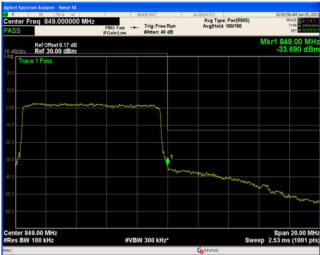
Band7 QPSK BW=5MHz Channel=20775 RB Size=1 Position=#0
