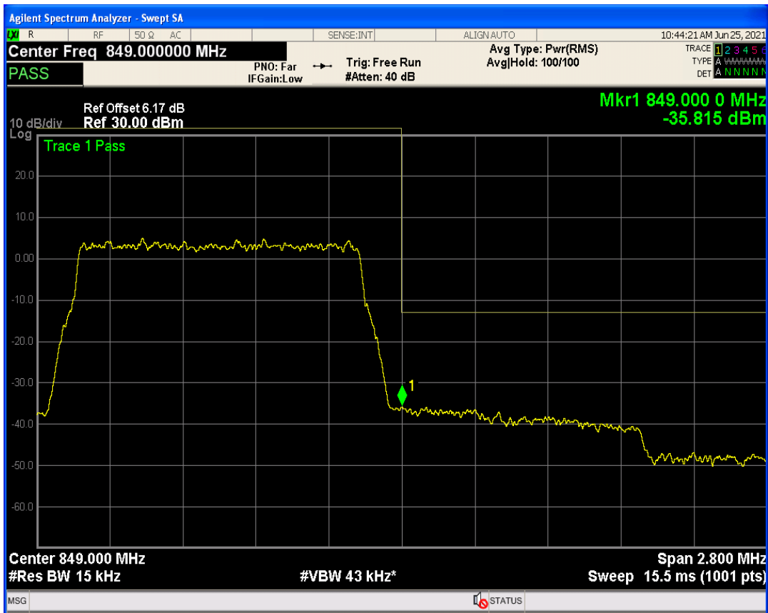
Band5 QAM16 BW=1.4MHz Channel=20643 RB Size=1 Position=#0
