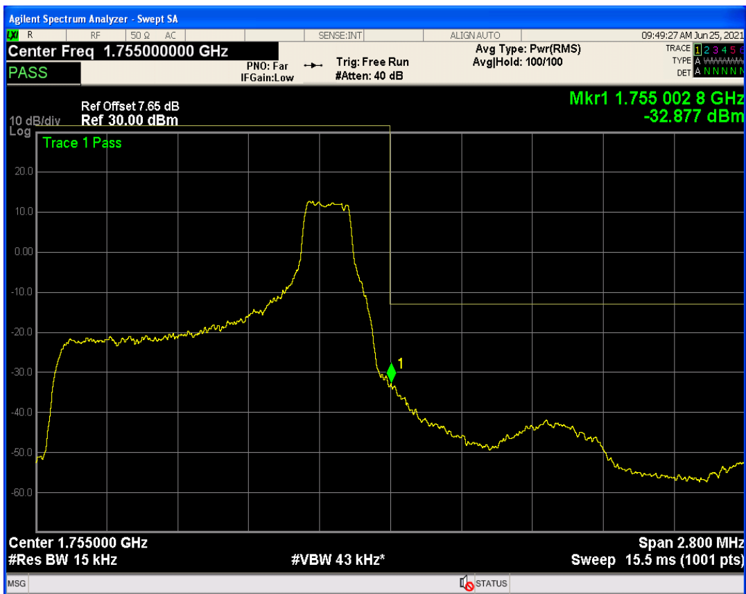
Band4 QPSK BW=3MHz Channel=19965 RB Size=1 Position=#Max
