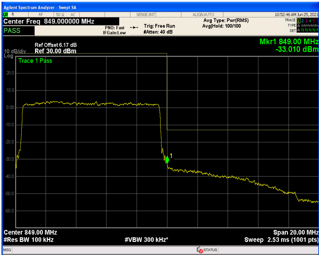
Band5 QAM16 BW=10MHz Channel=20600 RB Size=1 Position=#0
