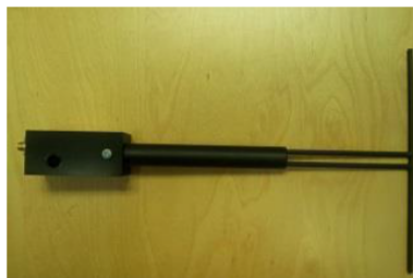
Figure 1 – MVG COMOSAR Validation Dipole
