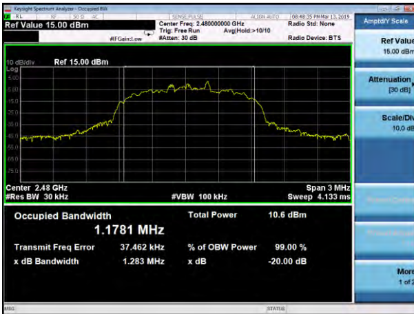
20dB Bandwidth plot on channel 78 (3Mbps)
