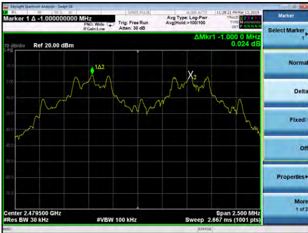
(1Mbps) Channel Separation plot on channel 77-78
