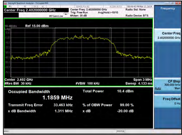
20dB Bandwidth plot on channel 39 (2Mbps)
