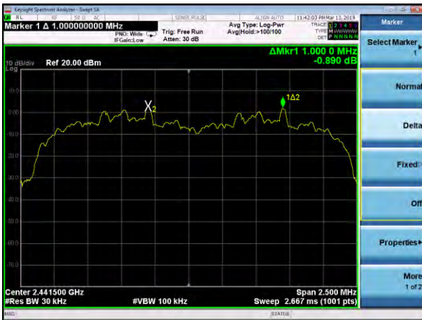
(3Mbps) Channel Separation plot on channel 39-40
