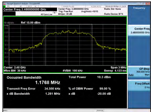
20dB Bandwidth plot on channel 78 (2Mbps)
