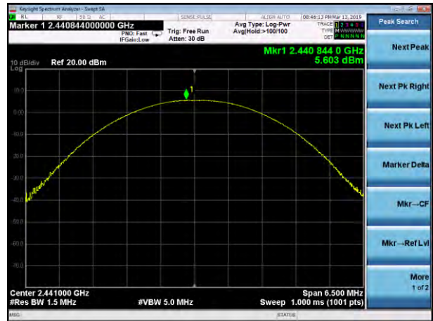
Peak output Power plot on channel 78 (2Mbps)
