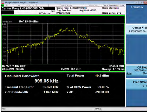
20dB Bandwidth plot on channel 39 (1Mbps)
