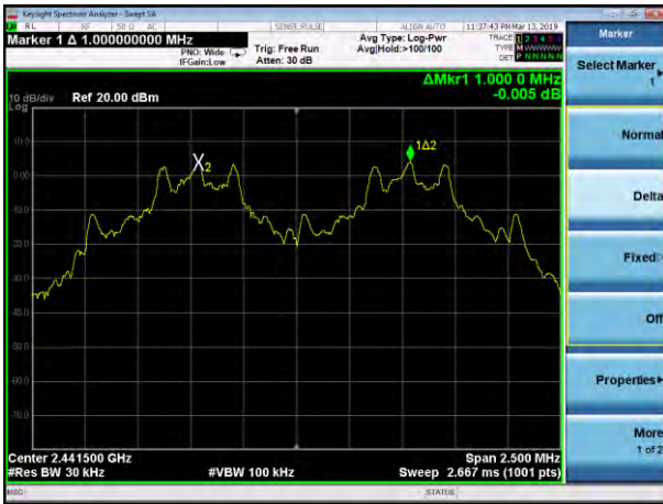
(1Mbps) Channel Separation plot on channel 77-78
