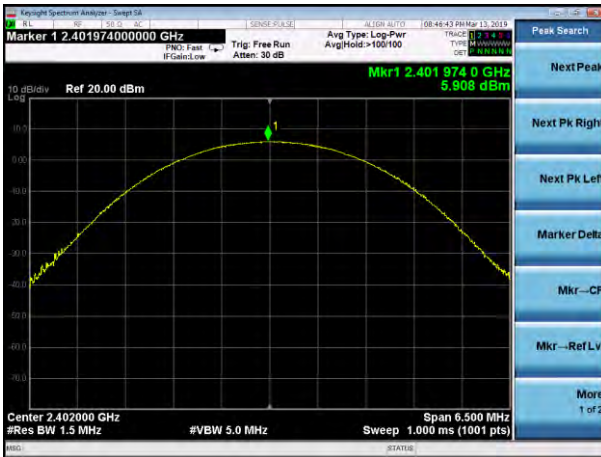
Peak output Power plot on channel 00 (3Mbps)
