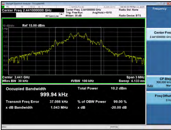
20dB Bandwidth plot on channel 78 (1Mbps)
