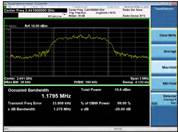
20dB Bandwidth plot on channel 78 (2Mbps)
