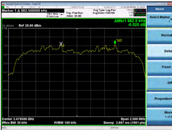
(3Mbps) Channel Separation plot on channel 77-78
