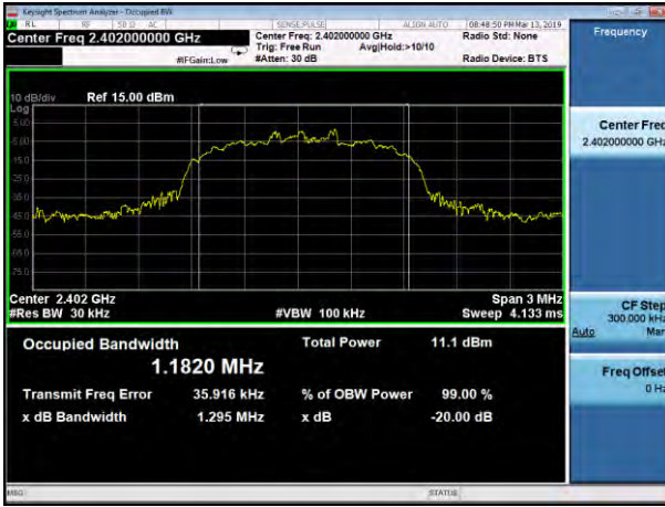
20dB Bandwidth plot on channel 39 (3Mbps)
