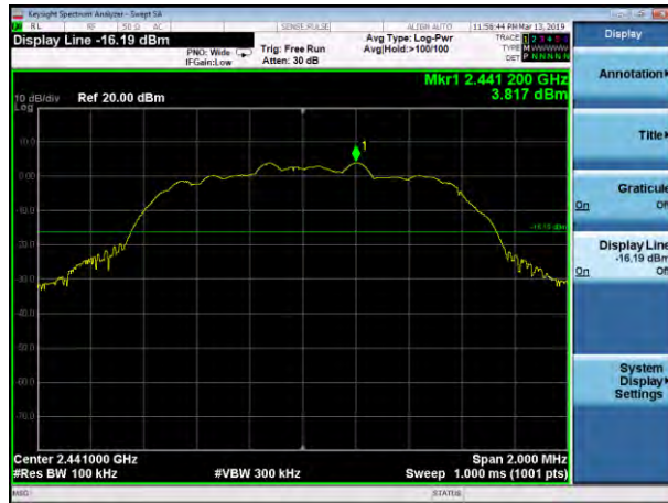
8-DPSK on channel 39
