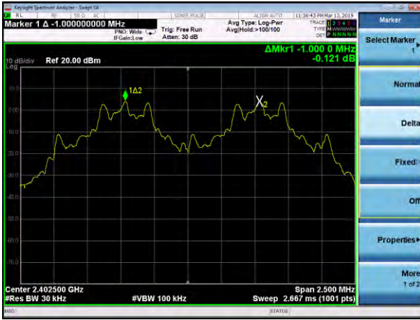
(1Mbps) Channel Separation plot on channel 39-40
