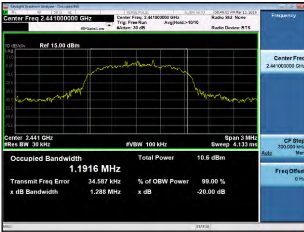
20dB Bandwidth plot on channel 78 (3Mbps)
