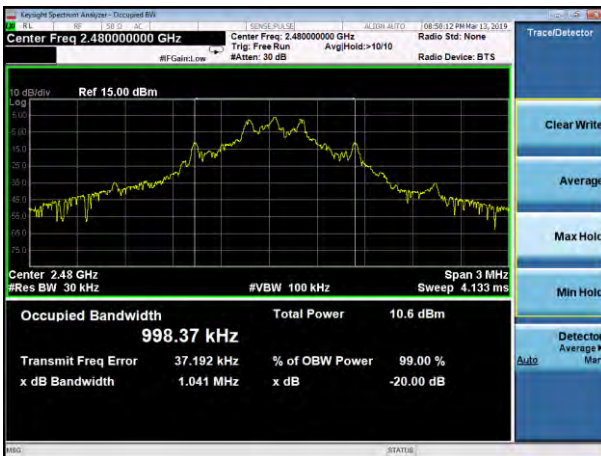
20dB Bandwidth plot on channel 78 (1Mbps)
