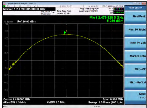
Peak output Power plot on channel 78 (2Mbps)
