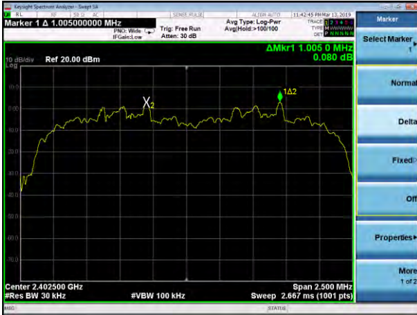
(3Mbps) Channel Separation plot on channel 39-40
