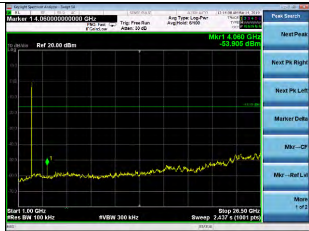
8-DPSK on channel 39
