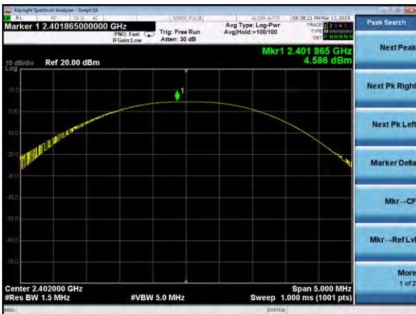
Peak output Power plot on channel 78 (1Mbps)
