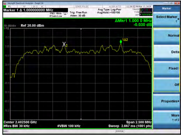
(2Mbps) Channel Separation plot on channel 39-40
