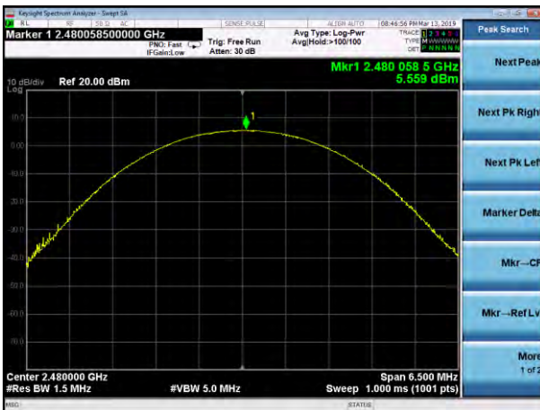
Peak output Power plot on channel 78 (3Mbps)
