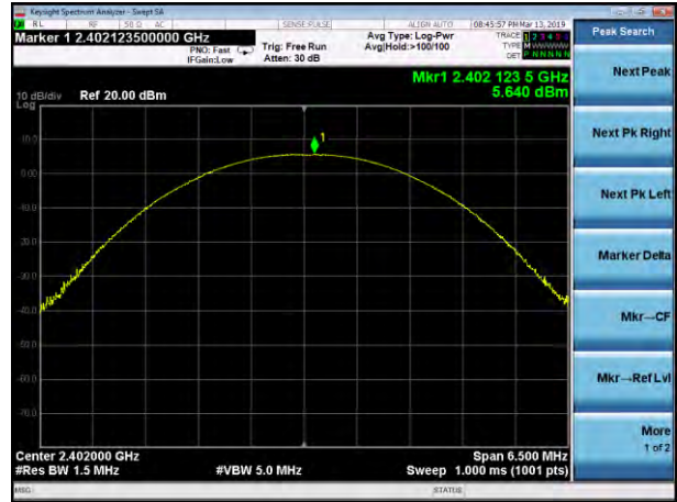
Peak output Power plot on channel 00 (2Mbps)
