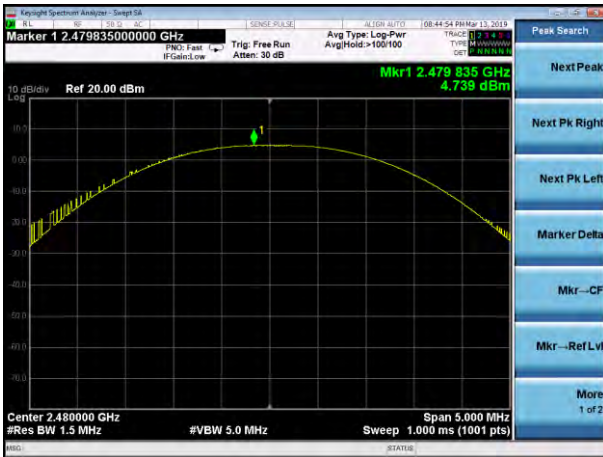
Peak output Power plot on channel 78 (1Mbps)
