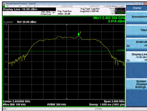
8-DPSK on channel 00
