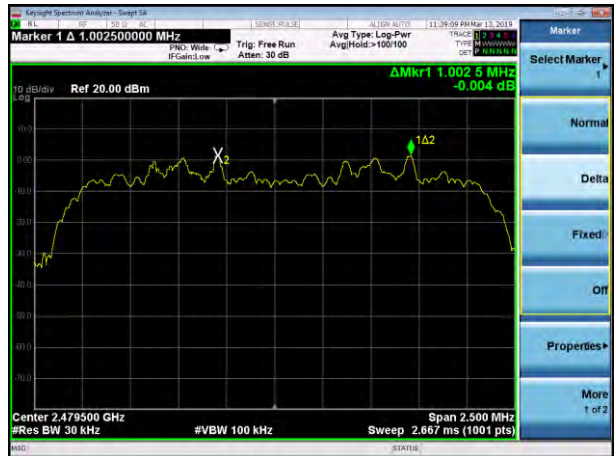
(2Mbps) Channel Separation plot on channel 77-78
