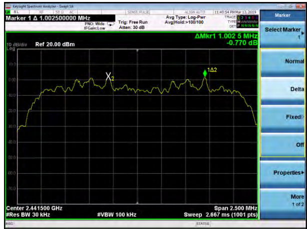
(2Mbps) Channel Separation plot on channel 77-78
