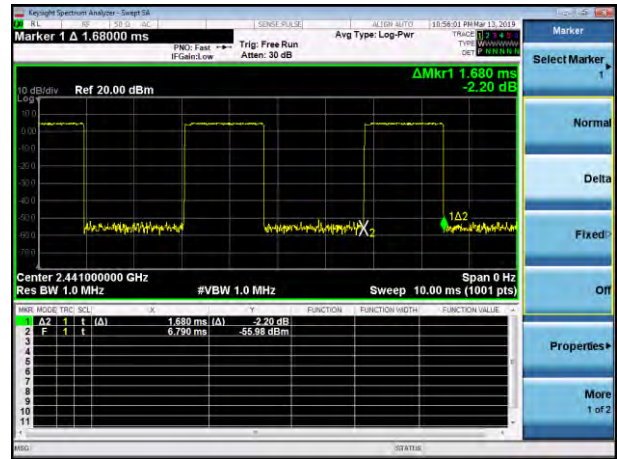
Package Transfer Time Plot CH39-2DH5
