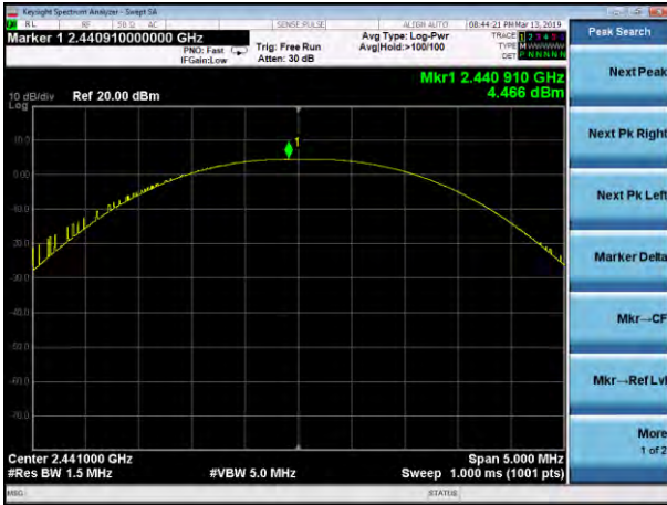
Peak output Power plot on channel 00 (1Mbps)
