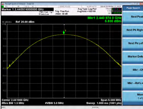
Peak output Power plot on channel 39 (3Mbps)
