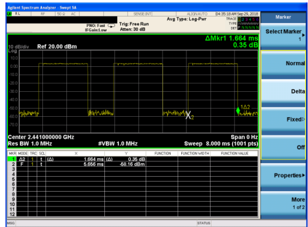
Package Transfer Time Plot CH39-2DH5
