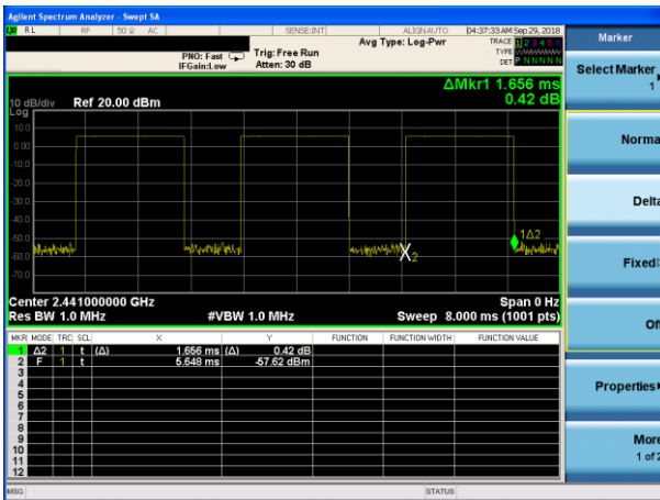
Package Transfer Time Plot CH39-DH5
