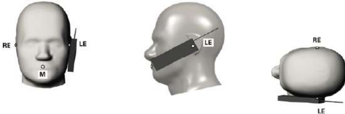
Fig. 11.3 Illustration for Cheek Position
