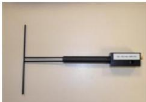
Figure 1 – Satimo COMOSAR Validation Dipole
