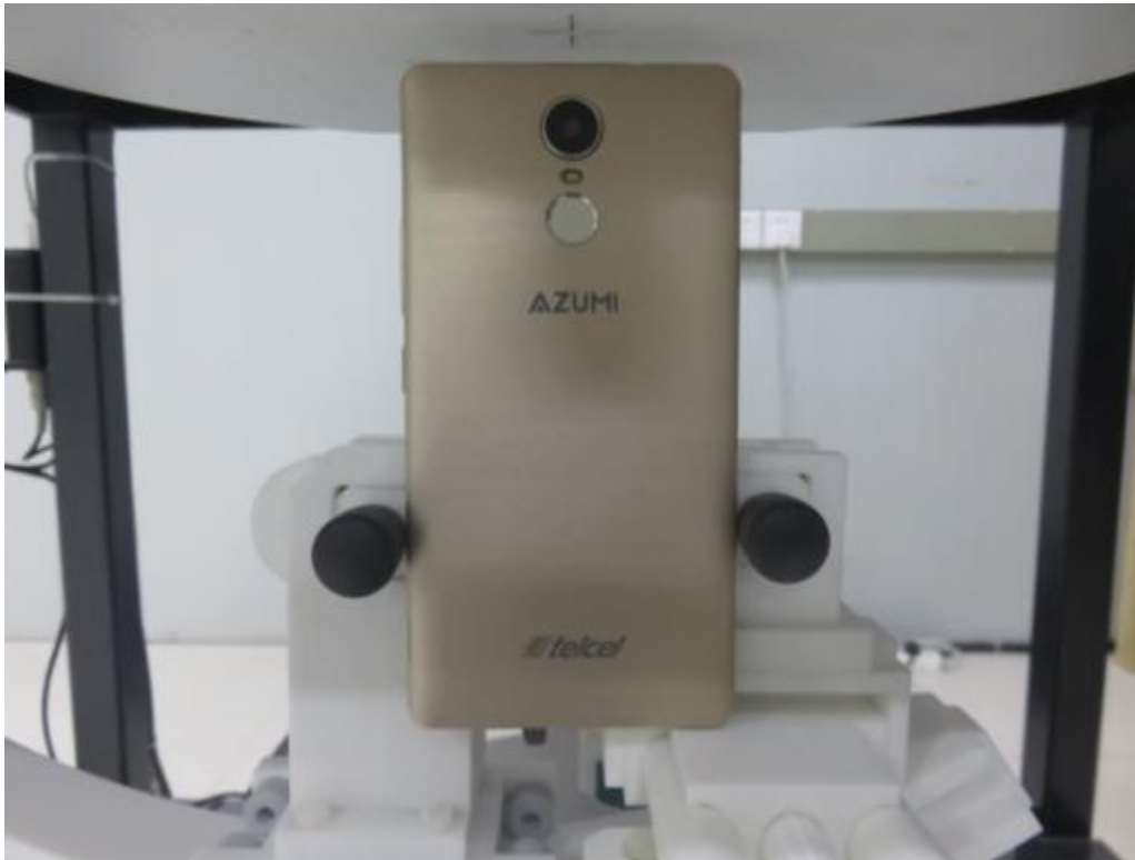
10mm body-worn Top Side Setup Photo(hotspot)
