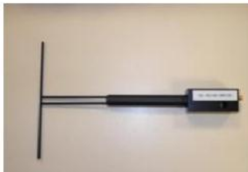
Figure 1 – Satimo COMOSAR Validation Dipole
