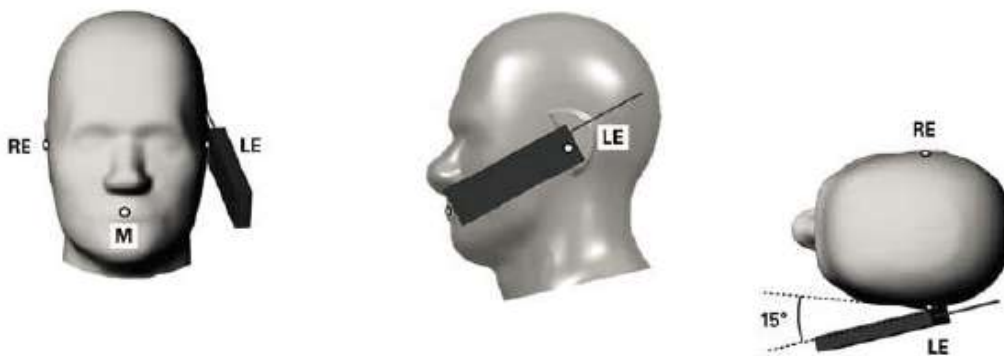
Fig.11.4 Illustration for Tilted Position
