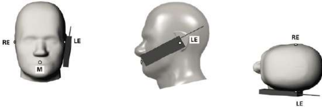
Fig. 11.3 Illustration for Cheek Position
