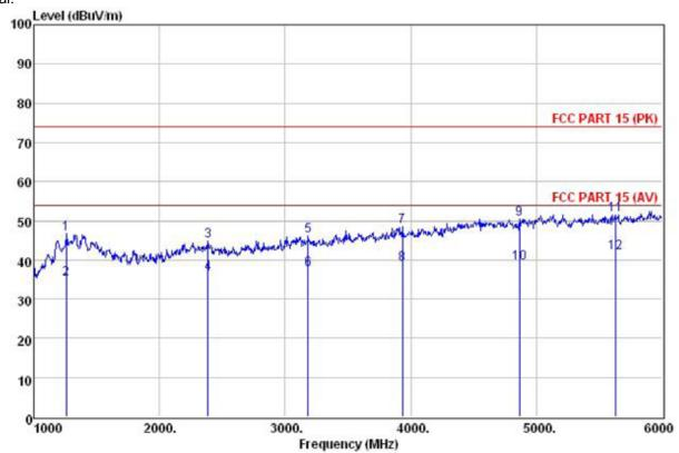
Site Condition 3m chamber FCC PART 15 (PK) 3m BBHA9120(>1GHZ) VERTICAL 204RF
