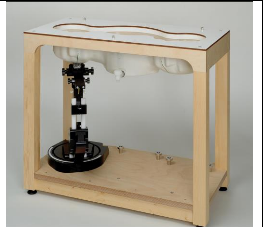
Fig. 8.7 Photo of SAM Twin Phantom
