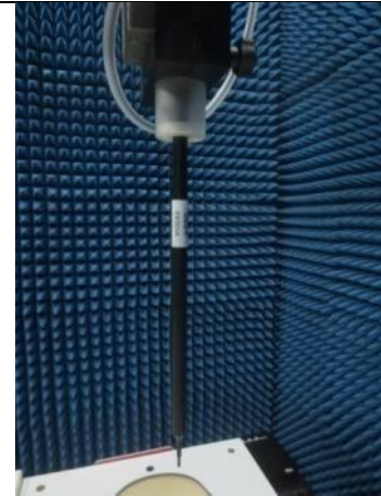
Fig. 8.2 Photo of E-Field Probe
