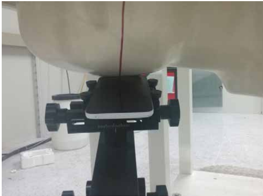
Right Head (EUT Tilted)
