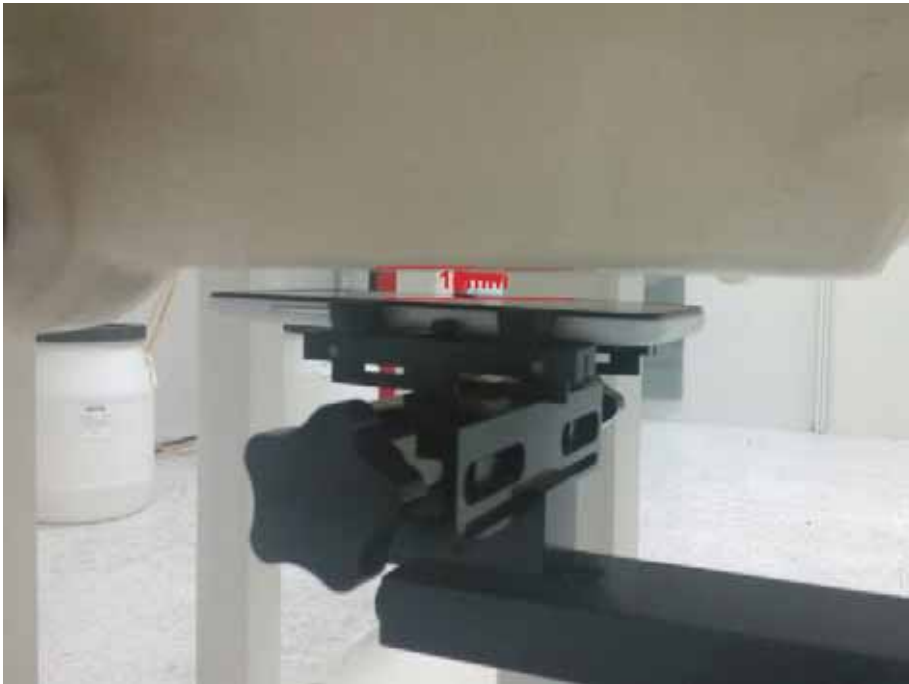
LTE Body Front at 10mm
