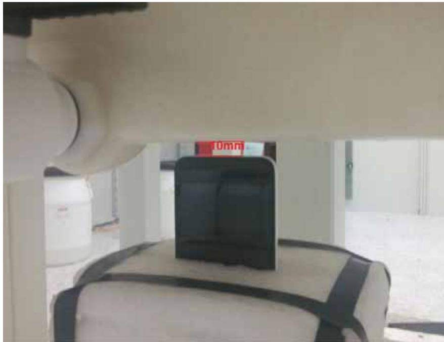
Body Top at 10mm WLAN
