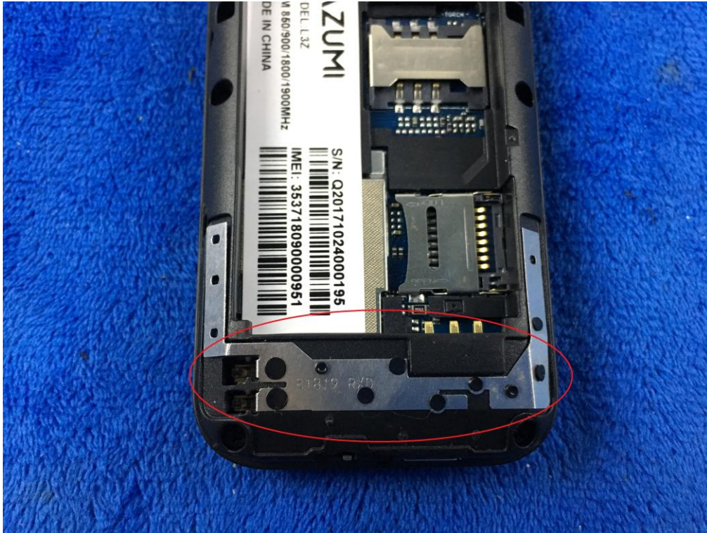
GSM/PCS Antenna View
