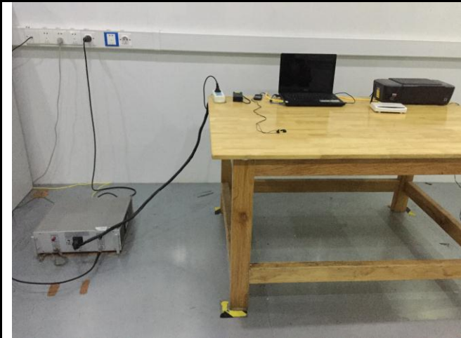
Conducted Emissions Test Setup – Front View
