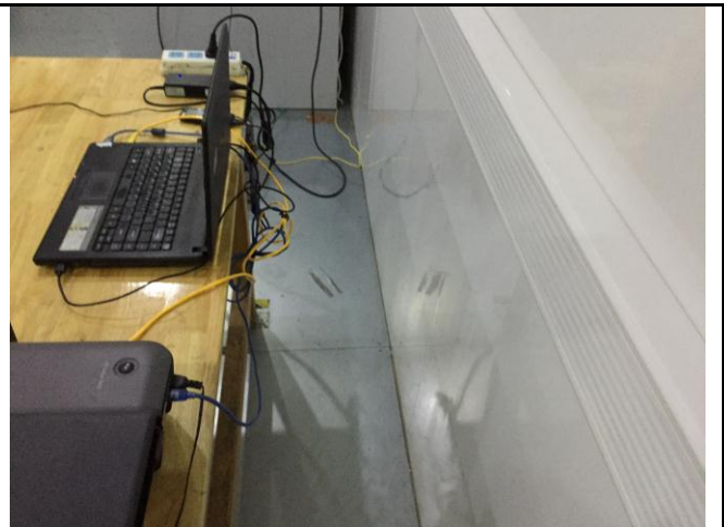
Conducted Emissions Test Setup – Side View
