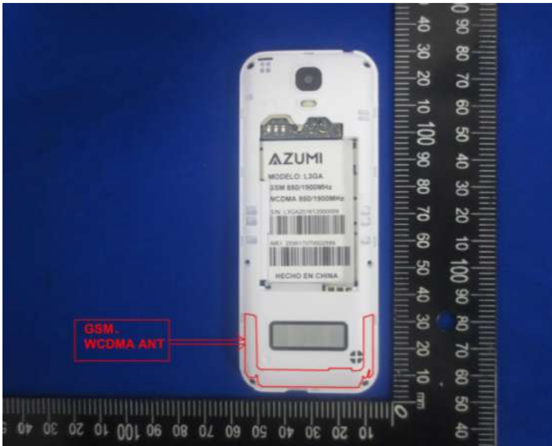
Fig.14.1 EUT Antenna Locations
