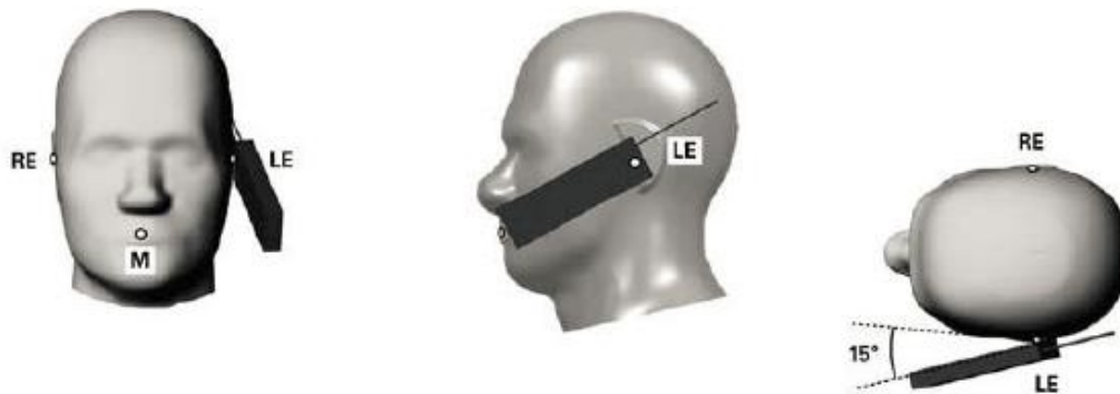
Fig.11.4 Illustration for Tilted Position
