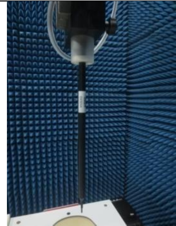
Fig. 8.2 Photo of E-Field Probe
