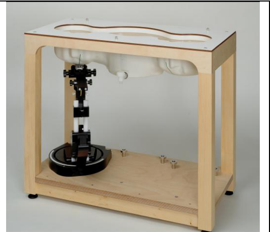
Fig. 8.7 Photo of SAM Twin Phantom
