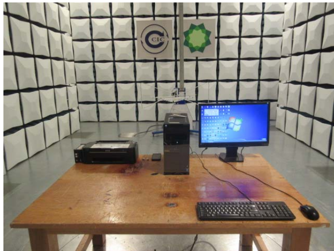
Radiated Emission (above 1GHz) Connect to PC
