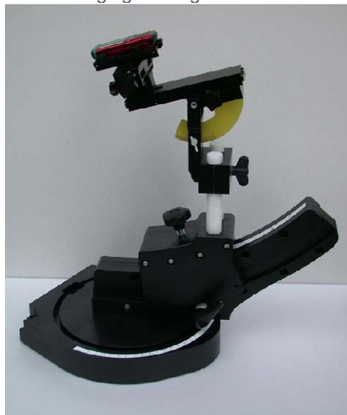
Device holder supplied by SPEAG
