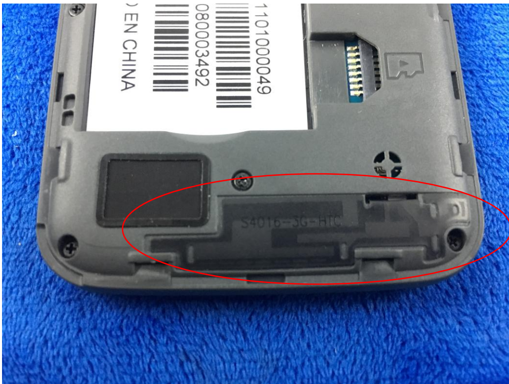
GSM/PCS/UMTS-FDD Antenna View
