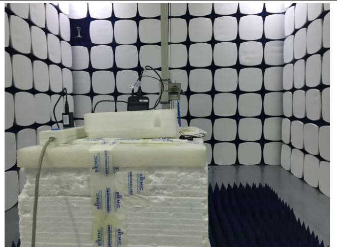
Radiated Spurious Emissions Test Setup Above 1GHz
