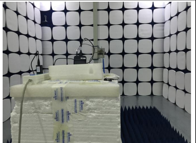
Radiated Spurious Emissions Test Setup Above 1GHz
